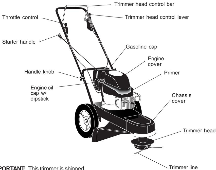
**IMPORTANT:** This trimmer is shipped WITHOUT OIL OR GASOLINE in the engine.
