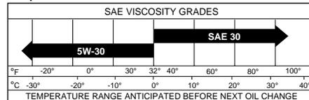
**NOTE:** Although multi-viscosity oils (5W30, 10W30 etc.) improve starting in cold weather, these multi-viscosity oils will result in increased oil consumption when used above 32°F. Check your engine oil level more frequently to avoid possible engine damage from running low on oil.
