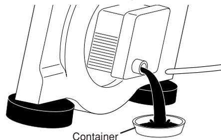
5. Slowly pour oil down the oil fill spout, stopping every few ounces to check the oil level with the dipstick.
